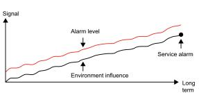
Reliable operation is ensured as the alarm limit of the analogue smoke detector is self compensating, i.e. it will always remain at the correct preset value due to the built-in intelligence compensating for environmental changes.
