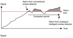
The analogue smoke detector controls the alarm signals from smoke in it's chamber by measuring time, amplitude of signal and signal spread. Before transmitting a fire signal the smoke value must conform with preset data.
